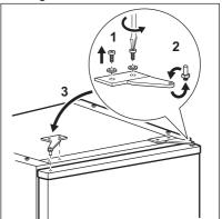
9. Remove the hinge. Put over the pin in the direction of the arrow. Install the hinge on the opposite side.
