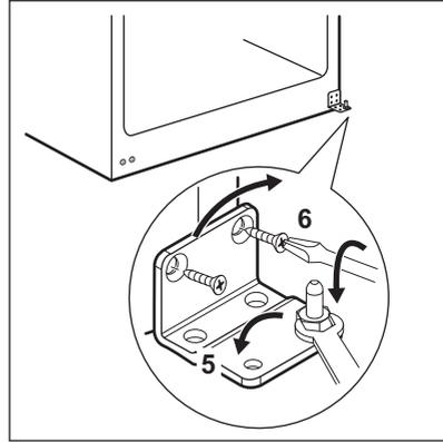
9. Screw off the screws of the lower hinge and remove the hinge (8).
