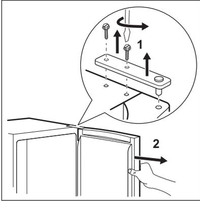
3. Remove the door from the middle hinge pivot (2).
