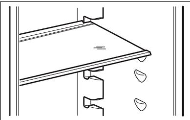
The walls of the refrigerator are equipped with a series of supports so that the shelves can be positioned as desired.
