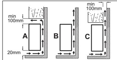
In order to guarantee proper functioning in ambient temperature above 38°C, it is advised to have a 30mm separation between the sides of the appliance and surrounding furniture.
